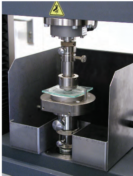
A puncture testing setup includes a collection tray to capture broken glass
