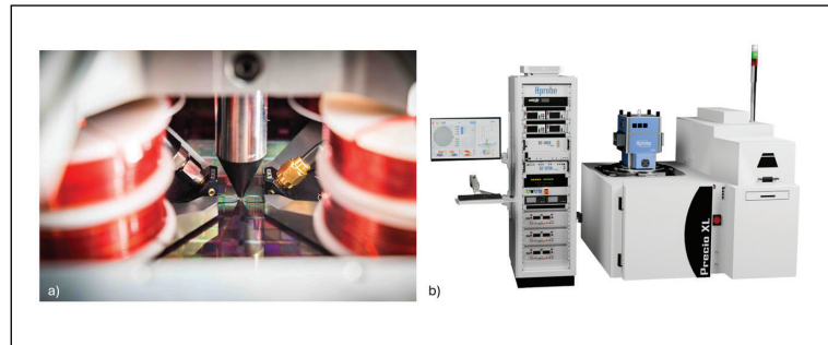
➤ Figure 1: a) Inside the Hprobe Test Head: Magnetic Field Generation and Wafer-Level Probing b) Hprobe ATE integrated with TEL Precio XL wafer prober
