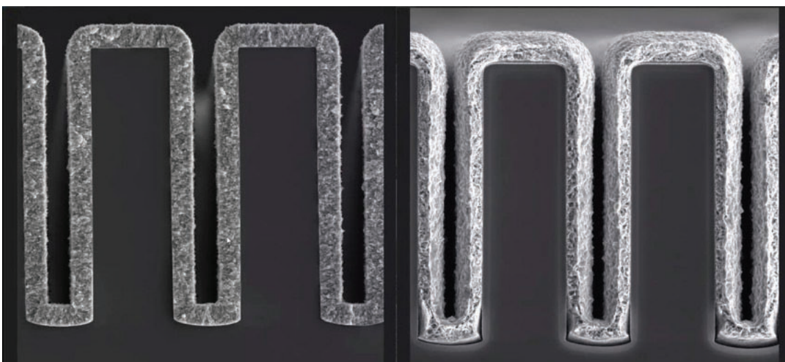
► Figure 3. Copper electrodeposition in 4:1 AR blind silicon vias utilizing (left) ALD-coated SiO 2 /TiN/Ru barrier/seed and (right) PVD-coated Ti/W barrier/seed. Numerous voids, trench narrowing and bread-loafing is visible when plating on a PVD seed layer.
