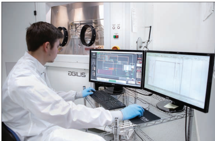
The Imperium-MOCVD software from Agnitron was built with TwinCAT 3 automation software from Beckhoff, and relies on the ability to program the machine logic in C# using Microsoft Visual Studio.
