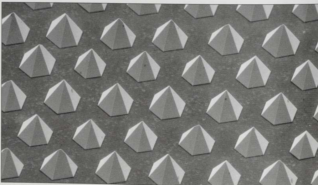
Figure 2: SEM picture of a GaN field emitter array fabricated at NCSU by O. H. Nam and R.F. Davis of NCSU. Peak to peak distance between pyramids is 10 \mu m. This surprisingly regular and uniform pattern was formed not by etching, but by self-limiting selective epitaxy.
