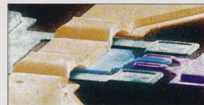
False color SEM of a InGaP/GaAs HBT. The small blue "finger" (center, right) is the emitter (measuring 3 \times 10 \mu\text{m}^2 ). The two adjacent fingers (pink) are the base contacts, and the two larger, outer fingers (green) are the collector contacts. A 2.5 \mu\text{m} Au evaporated airbridge emitter RF pad can be seen arching over the collector fingers. Image courtesy of the Semiconductor Research Group at the University of Illinois.
