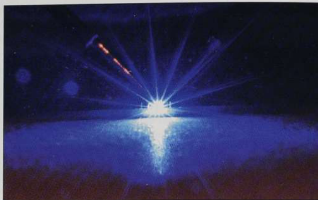
Edge emission from Cree's cleaved-facet InGaN/GaN MQW index guide laser diode grown on SiC.
