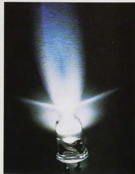
Figure Two. A white light "LUCOLED" LED produced by Siemens as a result of color conversion techniques developed at the Fraunhofer IAF. Siemens is expected to launch volume production sometime next year.
