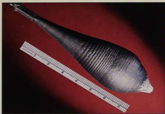
Figure One. An example of an InPAs ternary single crystal. These boules can typically be grown up to 2-3cm. diameter, 4-8cm long and 100-150gms in weight.
