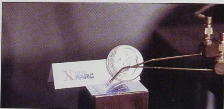
Figure Three. The latest blue laser. Xerox is unique in that it hopes to develop blue lasers for printing applications.
