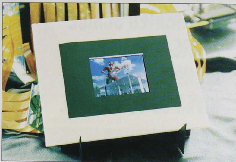
Figure 4. An Idemitsu Kosan full color quarter VGA OLED display (photo courtesy Dr. Tadashi Kusumoto, Idemitsu Kosan).
