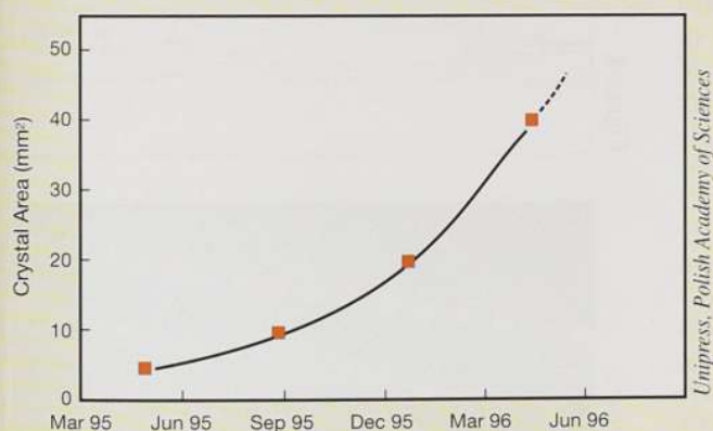
Figure One: Progress at Unipress in increasing GaN crystal size. Crystal area doubles every 3-4 months.
