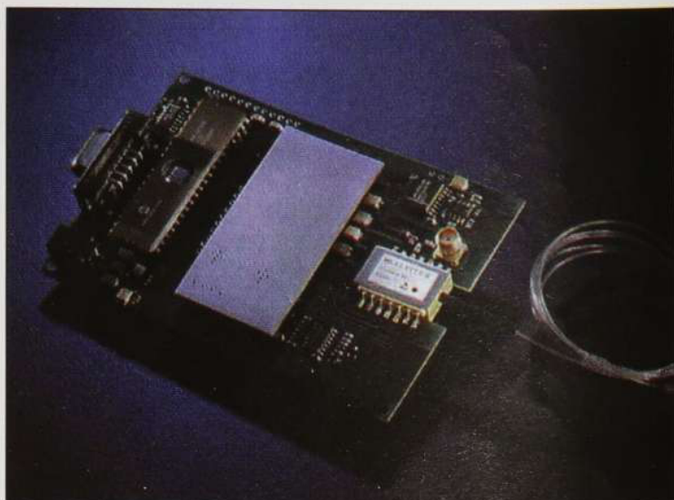
Altitud AB's tunable laser module mounted with controlling hardware.
