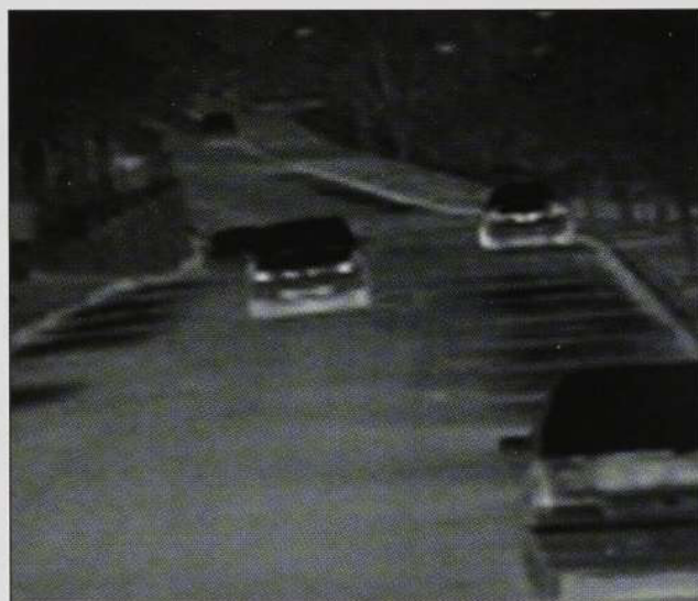
Figure 4: Image from a 640 \times 486 LWIR ( 8\text{--}9\text{ }\mu\text{m} ) QWIP staring array camera taken at around midnight. The places where cars were parked during the day are clearly visible as cooler, dark areas.
