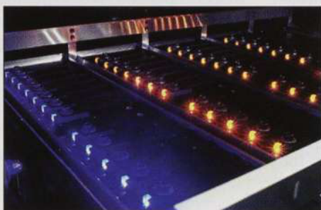
Testing of blue and yellow LEDs at Emcore.
