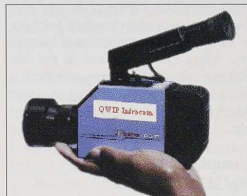
Figure 5: A palm-sized LWIR camera manufactured by Inframetrics incorporating a 256 \times 256 QWIP array made at JPL.
