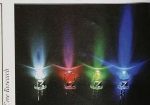
Examples of LUCOLEDs (luminescence conversion LEDs) developed at the Fraunhofer IAF.
