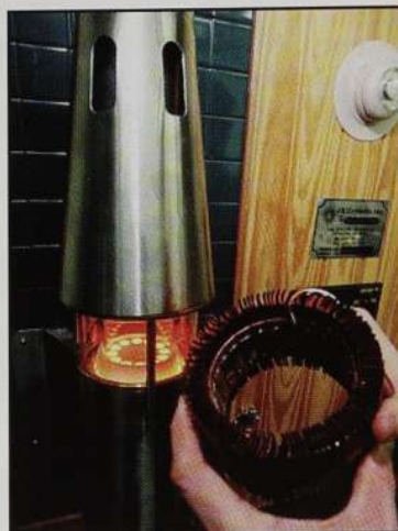
The 8,000 BTU/hour Midnight Sun unit burns propane to heat both its surroundings and the ceramic emitter. A cylindrical GaSb TPV array (shown in the photo with attached cooling fins) converts radiation from the emitter to produce 30 W electricity.
