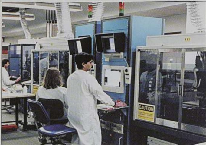
Figure 2. Lucent's MRC has localized cleanrooms operating from a single purge facility, creating a more relaxed and efficient working environment.
