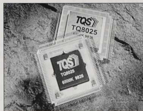
TriQuint's TQ8025 is a 16 x 16 digital crosspoint switch, for optical communication systems.
