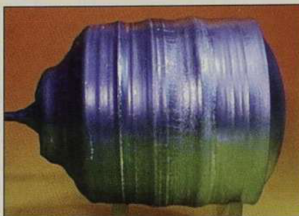
Figure 1: Typical 150mm S.I. GaAs LEC crystal grown at Freiberger. Presently, crystals with 160 ± 5mm in diameter and a bulk length of approximately 140mm are grown, allowing the manufacturing of >100 wafers per ingot.
