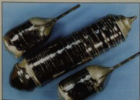
A new process for growing much longer 2" diameter InP crystals results in up to 250 wafers per ingot.
