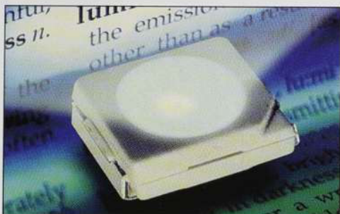
An example of a white light LED from Siemens. For more on these devices, see our "Things to Watch" feature, beginning on page 25.
