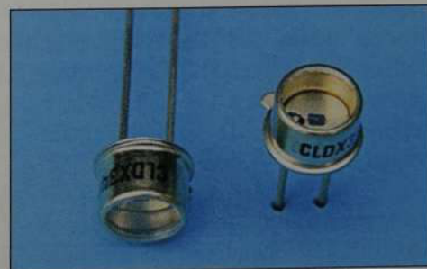
850 - 910 nm AlGaAs photodiode, capable of operating at 225°C.
