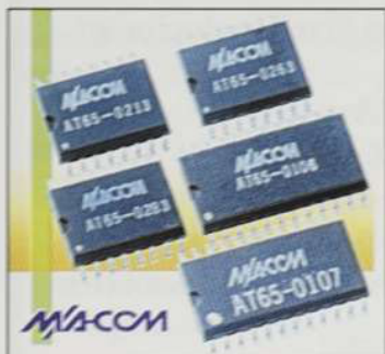
M/A-COM recently announced a family of digital attenuators with integral ASIC drivers, in surface mount multi-chip modules.
