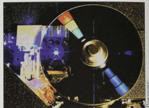
Matsushita's second harmonic generation (SHG) laser mounted onto an optical head to demonstrate the feasibility of high density recording and direct modulation.
