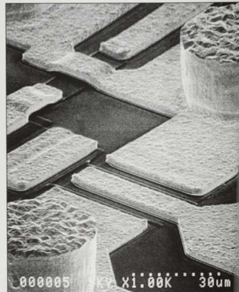
Figure 2. SEM image of a MMIC prior to flip-chip bonding, showing HEMTs and 40 \mu\text{m} diameter pillar-shaped gold interconnections.
