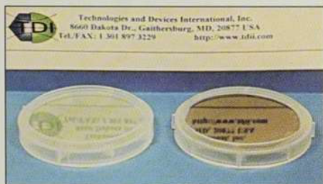
Figure 1. 2 inch 6H- and 4H-SiC epi wafer with reduced micropipe density.
