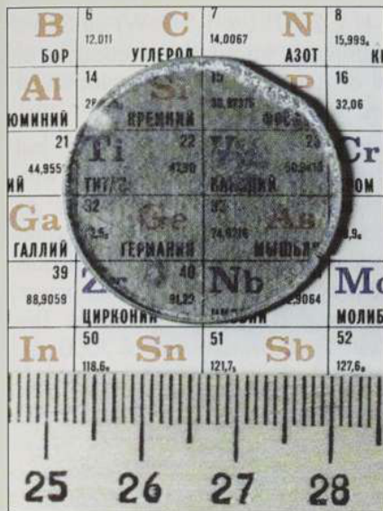
Figure 3. Free-standing 30 mm diameter GaN wafer fabricated by HVPE GaN growth on SiC substrate and subsequent substrate removal by reactive ion etching.
