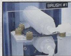
Patented double brush cleans top, bottom, and edge with no chuck marking.
