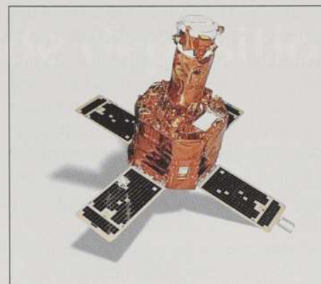
NASA's TRACE satellite, one of the spacecraft on which Tecstar's triple junction solar cells were successfully demonstrated.
