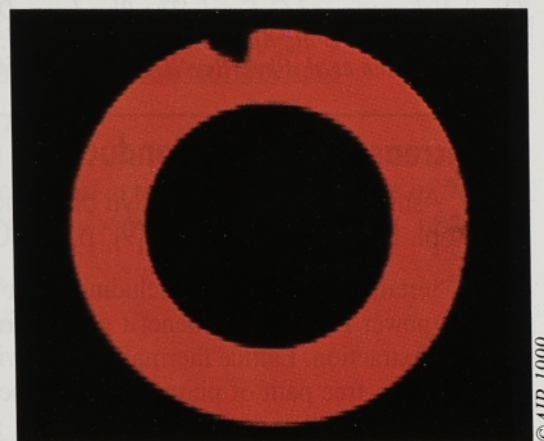
Photograph of red emission from a ring structure ITO/GaN:Eu LED of area 7.65 \times 10^{-4} \text{ cm}^2 and ring width 75 \mu\text{m} , operating with 50 V and 0.6 mA. The dark notch in the upper part of the ring is caused by the probe tip obscuring the emission.
