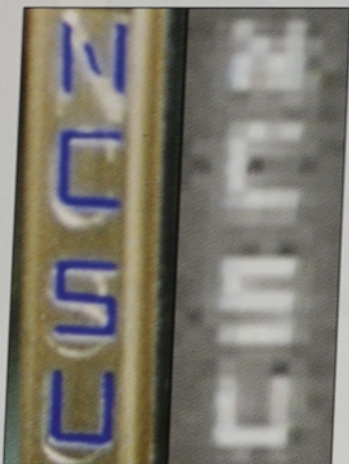
Figure 3. The UV source used to test the GaN/AlGaIn array (left), and the digital image without signal processing.
