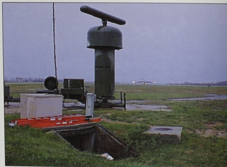
Figure 4. Portable MPN-25 X-band transmit/receive radar system used in military applications. Depending on the exact system, the active electronic scanned antenna can contain as many as a 1000 modules.
