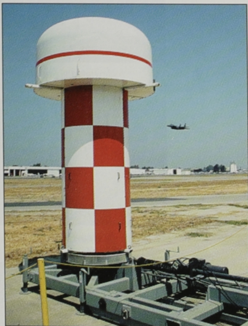
Figure 1. Ground Control Approach (PAR-2000) radar system produced by ITT's Gilfillan division. These systems are in use at several commercial airports and feature much increased safety as a result of the sheer number of modules contributing to radar detection.
