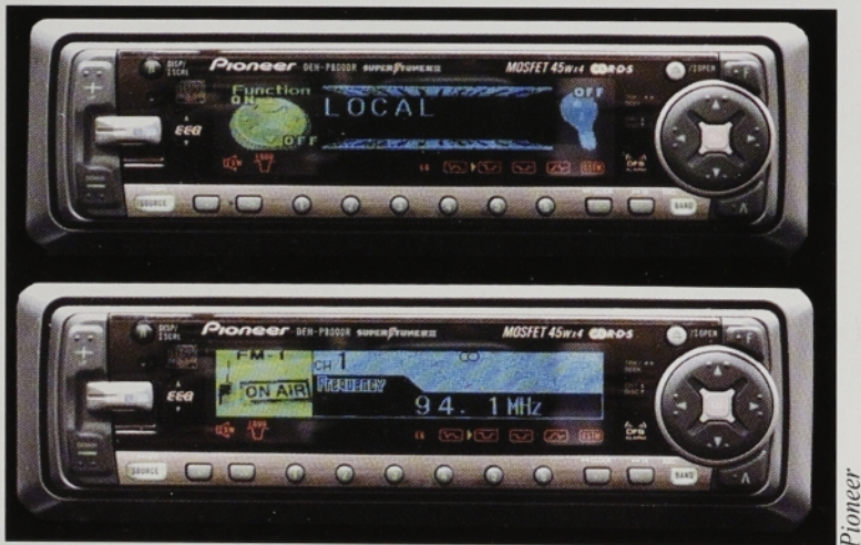
Figure 5. OEL display available from Pioneer. Based on Kodak's small molecule technology and using a passive matrix, the CD player went on sale earlier this year.
