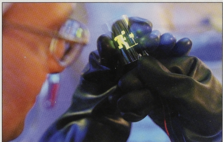
Figure 4. Siemens has developed flexible substrates for its displays. Its first product, expected next year, is a smart card with a flexible, bright OLED display. It also plans to offer passive matrix displays with high-performance power electronics in future.
