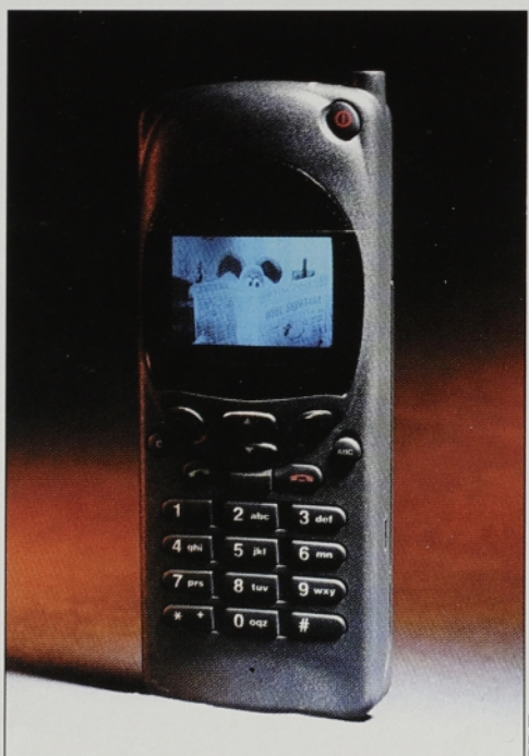
Figure 3. a) Side view of a monochrome, 2-inch video-rate active matrix display from CDT and Seiko-Epson. Unlike LCD or LED technology, OLEDs suffer no appreciable loss of intensity up to viewing angles of 170°. CDT has also developed polymers for color displays that use doping of blue to achieve green and red. b) Technology demonstrator developed by CDT and Seiko-Epson using active matrix technology for the display panel of a Nokia mobile phone.
