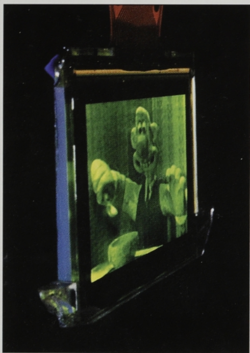
Figure 3. a) Side view of a monochrome, 2-inch video-rate active matrix display from CDT and Seiko-Epson. Unlike LCD or LED technology, OLEDs suffer no appreciable loss of intensity up to viewing angles of 170°. CDT has also developed polymers for color displays that use doping of blue to achieve green and red. b) Technology demonstrator developed by CDT and Seiko-Epson using active matrix technology for the display panel of a Nokia mobile phone.
