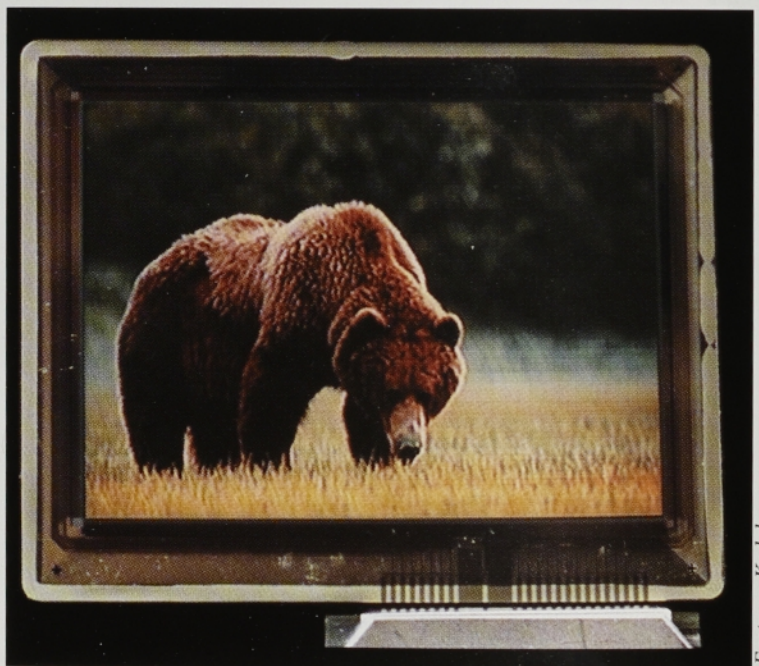
Figure 6. Video-rate, full-color OEL screen from Sanyo and Kodak. The screen is 2.4 inches across the diagonal and contains an 852 x 222 active pixel display. At 1.8 mm thick, it weighs less than its LCD counterpart, needs no backlight and consumes less power.
