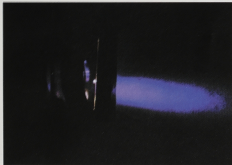
Figure 3. Color photograph of the violet beam emerging from an MQW InGaIn VCSEL cavity, showing a narrow radiation angle of approximately 5°.
