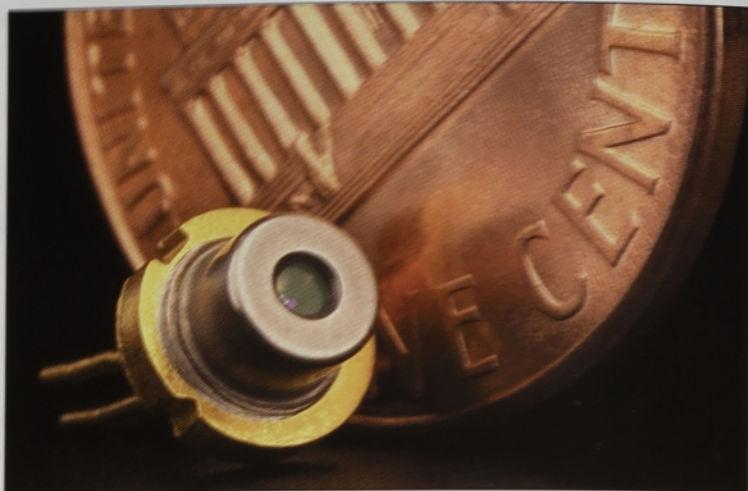
Figure 2. A tunable diode laser in a TO can package next to a U.S. one cent coin.
