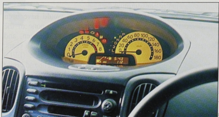
Figure 3. Dashboard panel featuring user-selectable color backlighting, which is also being employed for small cell phone displays.
