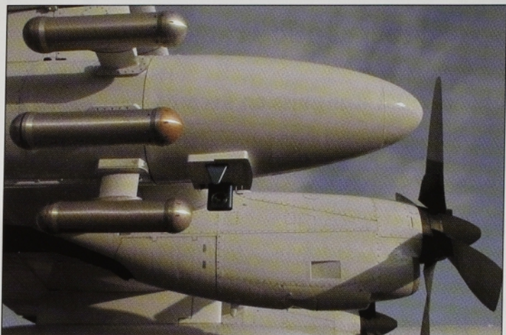
Figure 4. SpectraSensors' laser hygrometer shown mounted on NCAR's C-130 research aircraft.
