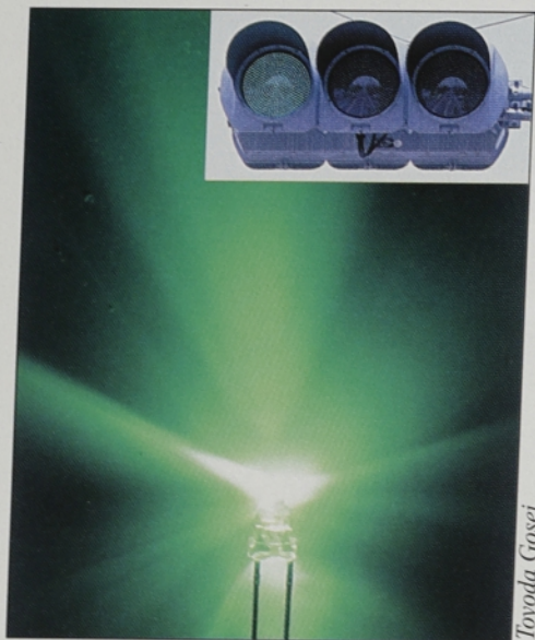
Figure 1. Toyoda Gosei's new high-brightness blue and green LEDs feature an inverted flip-chip design. This reduces total internal reflections and allows more light (up to 14 cd for the green device) to escape through the transparent sapphire substrate, making the LEDs very suitable for applications such as traffic lights.
