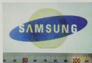
Figure 3. A 1.5-inch-diameter free standing GaN substrate grown by HVPE.
