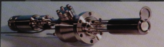
6 cc MINICELL (1 500°C) WITH SHUTTER AND WATER COOLING ON DN40CF (70 mm) FLANGE.
