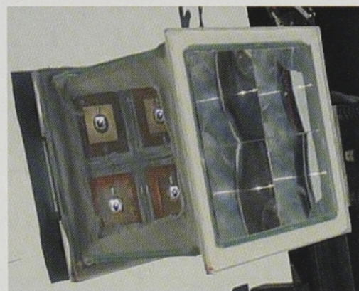
Figure 6. A small (64 cm 2 ) concentrator system with four \text{Ga}_{0.35}\text{In}_{0.65}\text{P}/\text{Ga}_{0.83}\text{In}_{0.17}\text{As} tandem solar cells working at a concentration ratio of 123.
