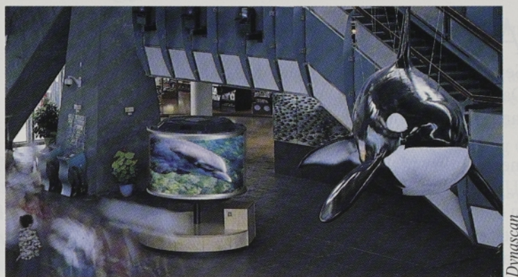
A 360° display manufactured by Dynascan uses only 21,600 LEDs to create three identical screens with a resolution of 864 × 480.
