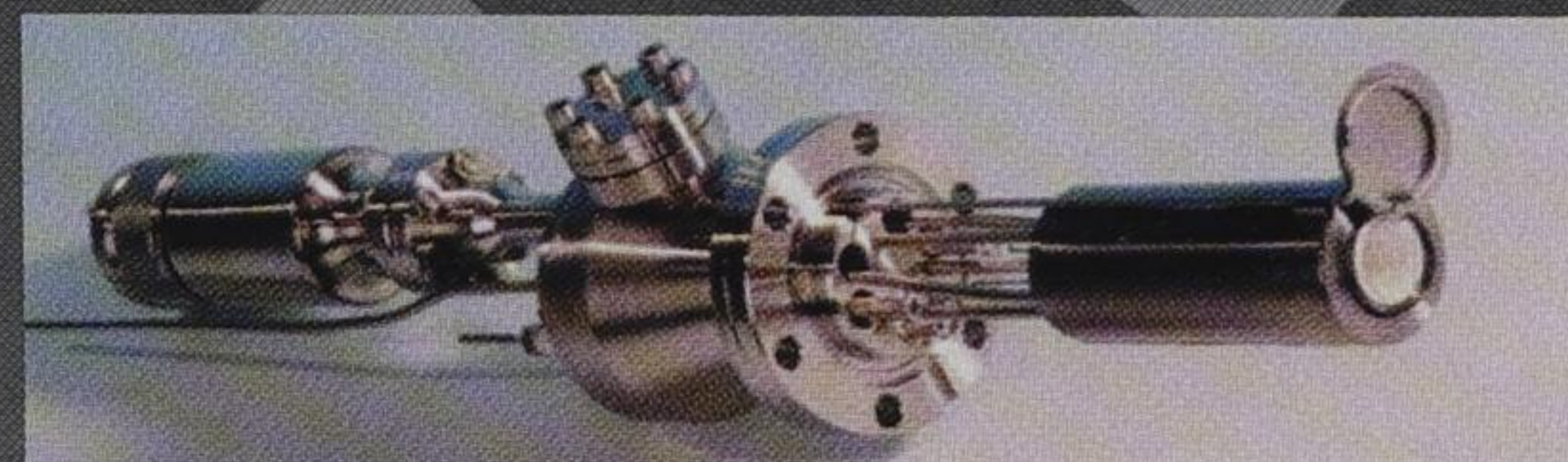
6 cc MINICELL (1 500°C) WITH SHUTTER AND WATER COOLING ON DN40CF (70 mm) FLANGE.
