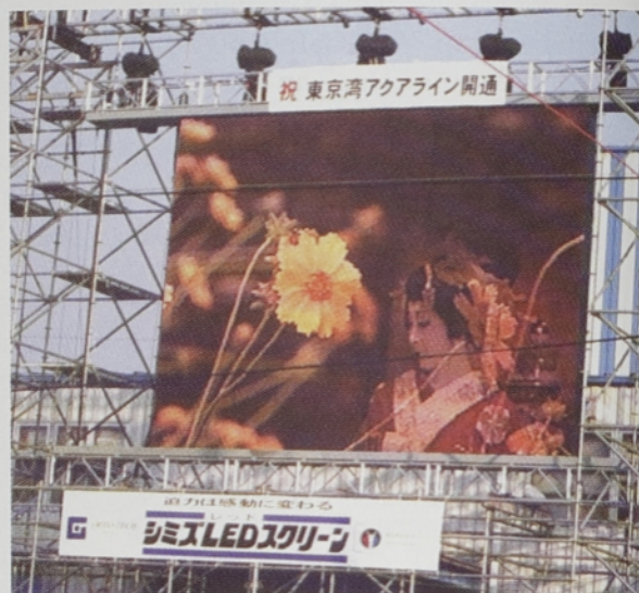
Full-color outdoor display manufactured by Opto Tech, composed of modules containing red, green and blue LEDs.
