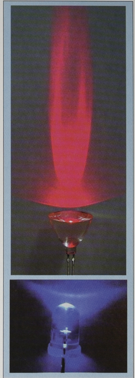
(top) Global Light's injection molding encapsulation process allows LEDs to be fabricated with unconventional shapes, as shown for this AlInGaP LED. (bottom) A conventionally shaped blue InGaP-based LED.
