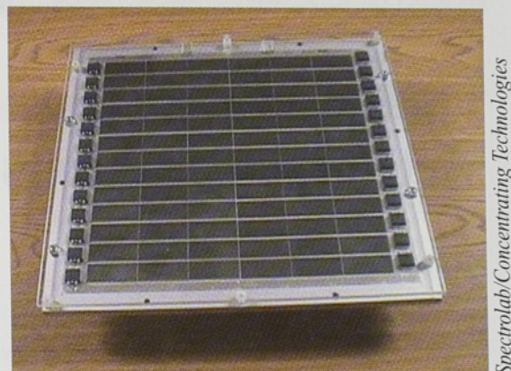
Figure 3. Dense array of GaInP/GaAs/Ge (triple-junction) solar cells made by Spectrolab. This ~20 × 20 cm 2 array will generate about 2.5 kW DC when Concentrating Technologies integrates it into a dish concentrator system, operating at ~ 250 suns.
