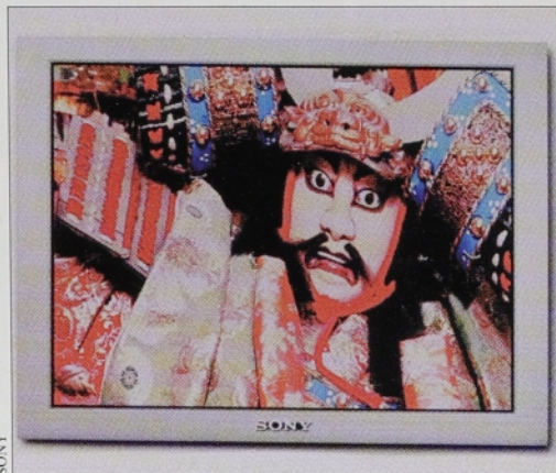
Sony's 13 inch OLED screen features a silicon TFT active matrix to drive the pixels, which are made from UDC's electro-phosphorescent organic light emitters.
