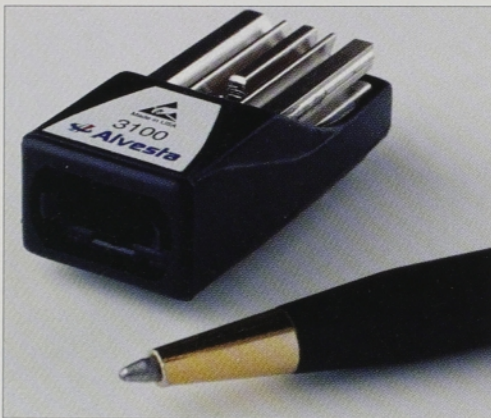
Fig. 1. Alvesta's four-channel parallel transceiver module contains arrays of four VCSELS and four detectors, and has a footprint of 0.61 × 1.36 inches.
