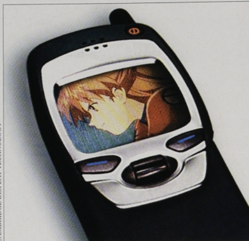
CDT's organic light emitters have been used by Seiko Epson to demonstrate a 30 000 pixel active matrix full-color cell phone display.
