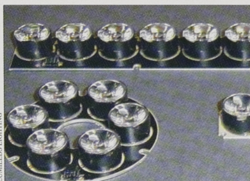
Line and Ring light sources employing LumiLeds' Luxeon LEDs.
