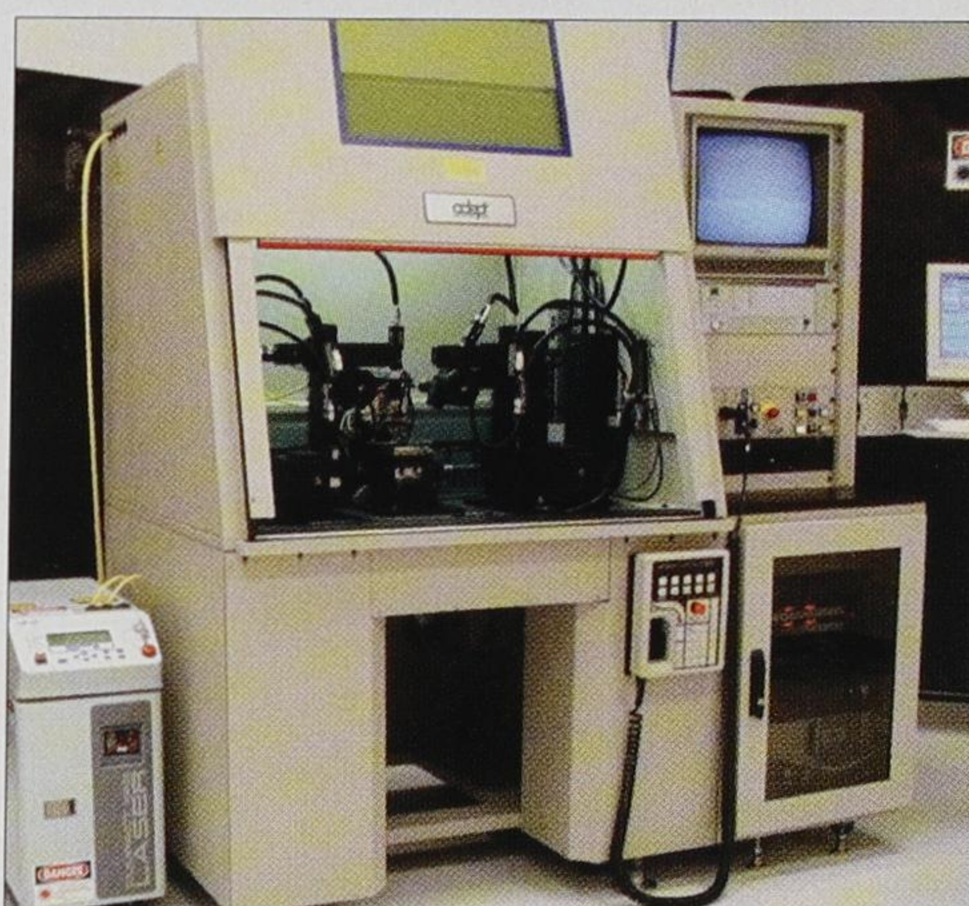
Fig. 1. An automated laser welding system manufactured by Adept Technology.
