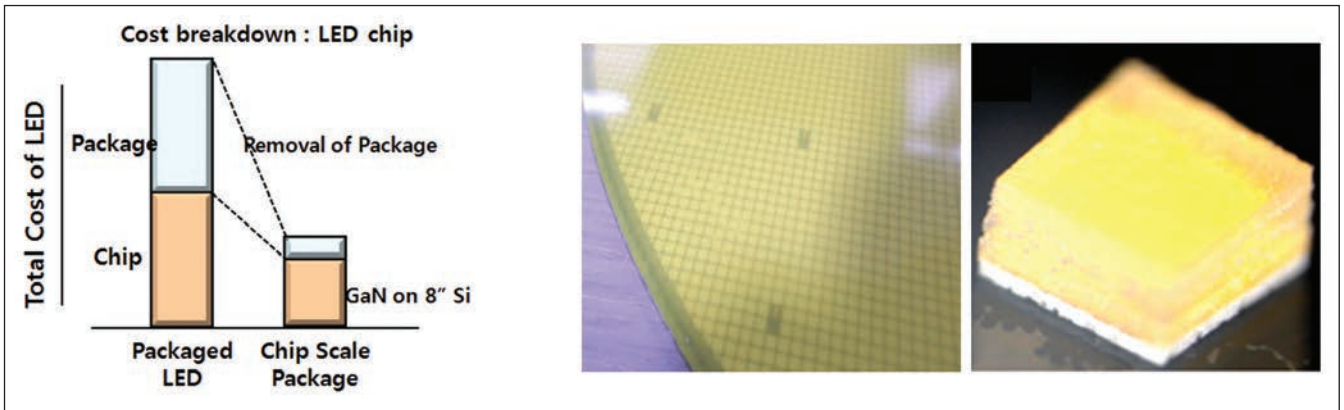
Figure 1. Switching to wafer-level, chip-scale packaging and 200 mm silicon substrates can slash the cost of the LED by 60 percent.
