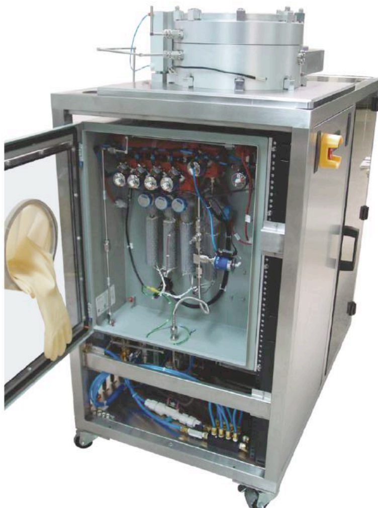
Precursors for the Nanomaster NLD-4000 are housed in a dedicated glove box.
