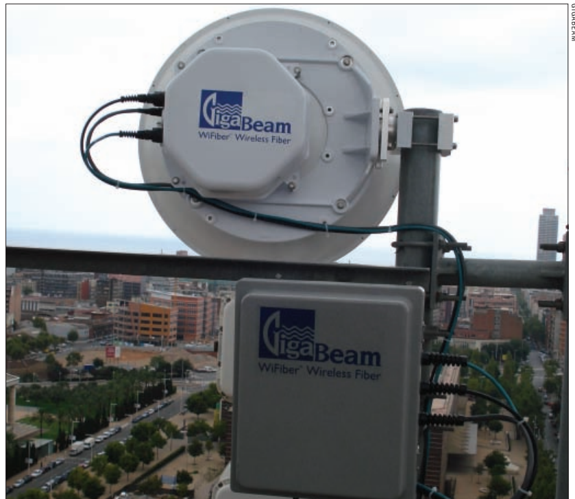
GigaBeam and its competitors , which build local high-speed wireless data links operating at 71–76 and 81–86 GHz, could benefit from HRL's powerful GaN MMICs. These devices can deliver an eight-fold improvement in power density over the equivalents built from InP and GaAs.
