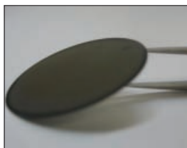
Group4 Labs is producing 2 inch GaN-on-diamond wafers that are sampled to customers and partners fabricating various forms of devices that generate heat.
