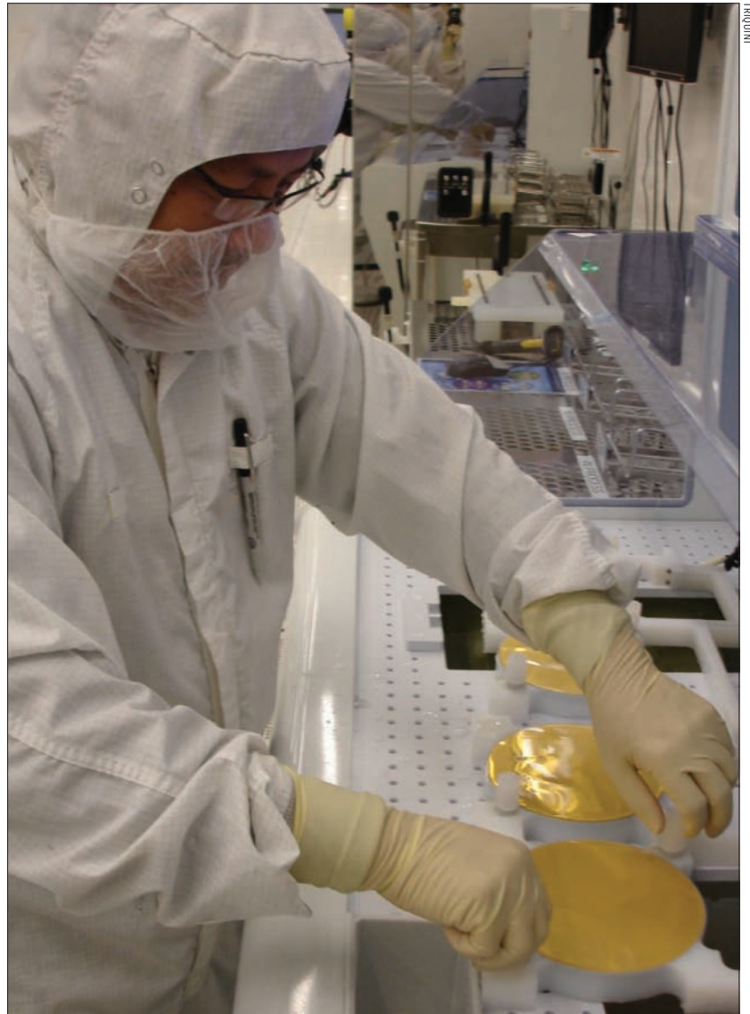
150 mm GaAs wafers being prepared for a gold-plating bath in TriQuint's Oregon fab. The company is addressing the demand for smaller devices with greater functionality with a BiHEMT process that combines HBTs and PHEMTs on one chip. This promises to unite power amplifiers with logic and bias control circuitry, low-noise amplifiers and ultimately antenna switches.
