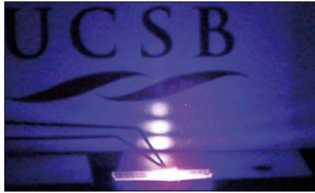
UCSB's first non-polar lasers use a broad-area design. The team plans to switch to a ridge-waveguide structure to reduce threshold current density.
