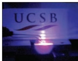
UCSB's first broad-area laser was announced this February. The initial device had a threshold-current density of 7.2 \text{ kA cm}^{-2} , but improvements to the design have already lowered this key figure of merit to 2.3 \text{ kA cm}^{-2} .
