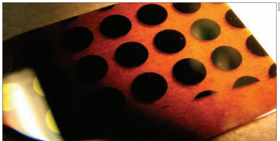
Green machine: using sunlight, chemical catalysts and commercial 2 inch GaP material, the UCSD team showed that carbon dioxide can be turned into a much more useful gas, carbon monoxide.
