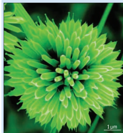
Fig. 2. A tin catalyst and process produce high-quality nanostructures (left and
