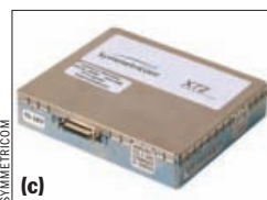
Fig. 1. Atomic clock evolution has improved portability: (a) NIST’s first cesium standard named NBS-1 from 1952; (b) Hewlett-Packard’s 5060A, which weighed 30 kg, from 1964; (c) Symmetricom’s model X72 rubidium oscillator; (d) Draper/Sandia MEMS physics package used in prototype CSACs.
