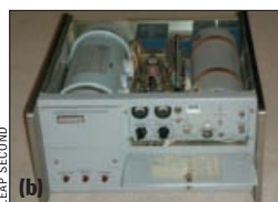
Fig. 1. Atomic clock evolution has improved portability: (a) NIST’s first cesium standard named NBS-1 from 1952; (b) Hewlett-Packard’s 5060A, which weighed 30 kg, from 1964; (c) Symmetricom’s model X72 rubidium oscillator; (d) Draper/Sandia MEMS physics package used in prototype CSACs.
