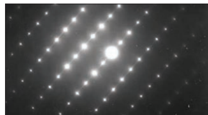
Fig. 1. (left) Nottingham's plasma-assisted MBE process can produce cubic GaN substrates of up to 50 \mu\text{m} in thickness with a surface area of more than 1 \text{cm}^2 . Fig. 2. (above) Reflection high-energy electron diffraction images of 30 \mu\text{m} thick free-standing GaN reveal the high quality of the cubic single-crystal structure.
