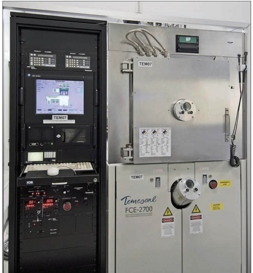
Skyworks Solutions has cut its PHEMT production costs by developing a new high-yield evaporation process that produces palladium barriers with a low gate-leakage current.
