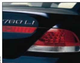
Conventional red LEDs are already used in car brake lights, but a switch to GaInPN devices could boost brightness or reduce the number of devices required.
