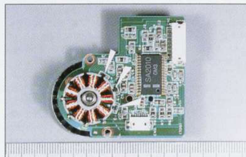
Figure 2: Photograph of a typical CD-ROM drive Hall motor showing three Hall elements (white arrows).
