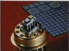
Figure 1. An integrated micro-TEC temperature controller (the gold block to the rear of the VCSEL) is available for wavelength stabilization or tuning (typically 0.06 nm/K).
