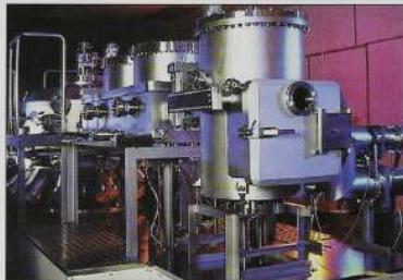
QED's V150 multiwafer MBE system - the industry's first multi-6" wafer MBE system.
