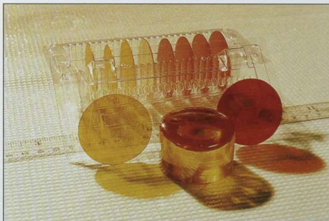
Eagle - Picher Beautiful, and rare - ZnSe substrates, grown by Eagle - Picher Industries.
