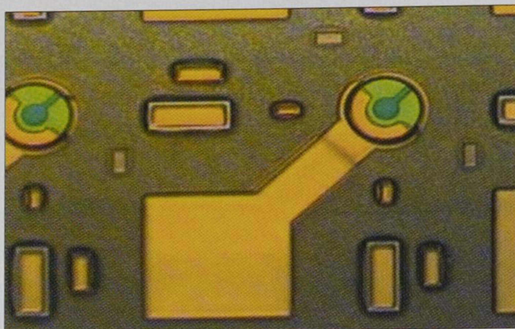
Fig. 2. An optical micrograph showing part of UEC's VCSEL array. Two lasers with 10 μm apertures that have been formed by oxide confinement are visible. The VCSELs are spaced at 250 μm intervals.
