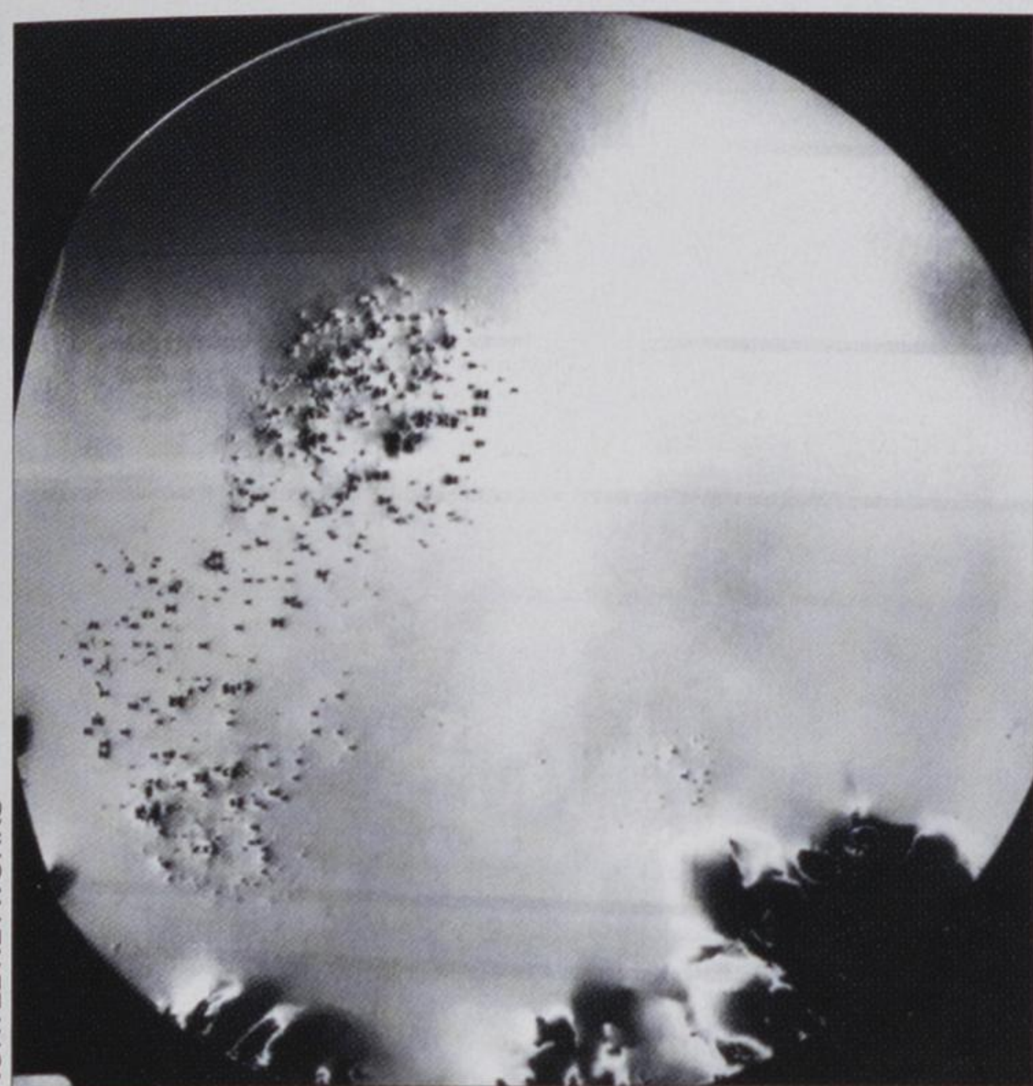
Fig. 3. Defects in a VGF-grown 4 inch InP(Fe) wafer are highlighted by asymmetric crystal x-ray topography. The map shows twinning, slip and slight polycrystallinity.
