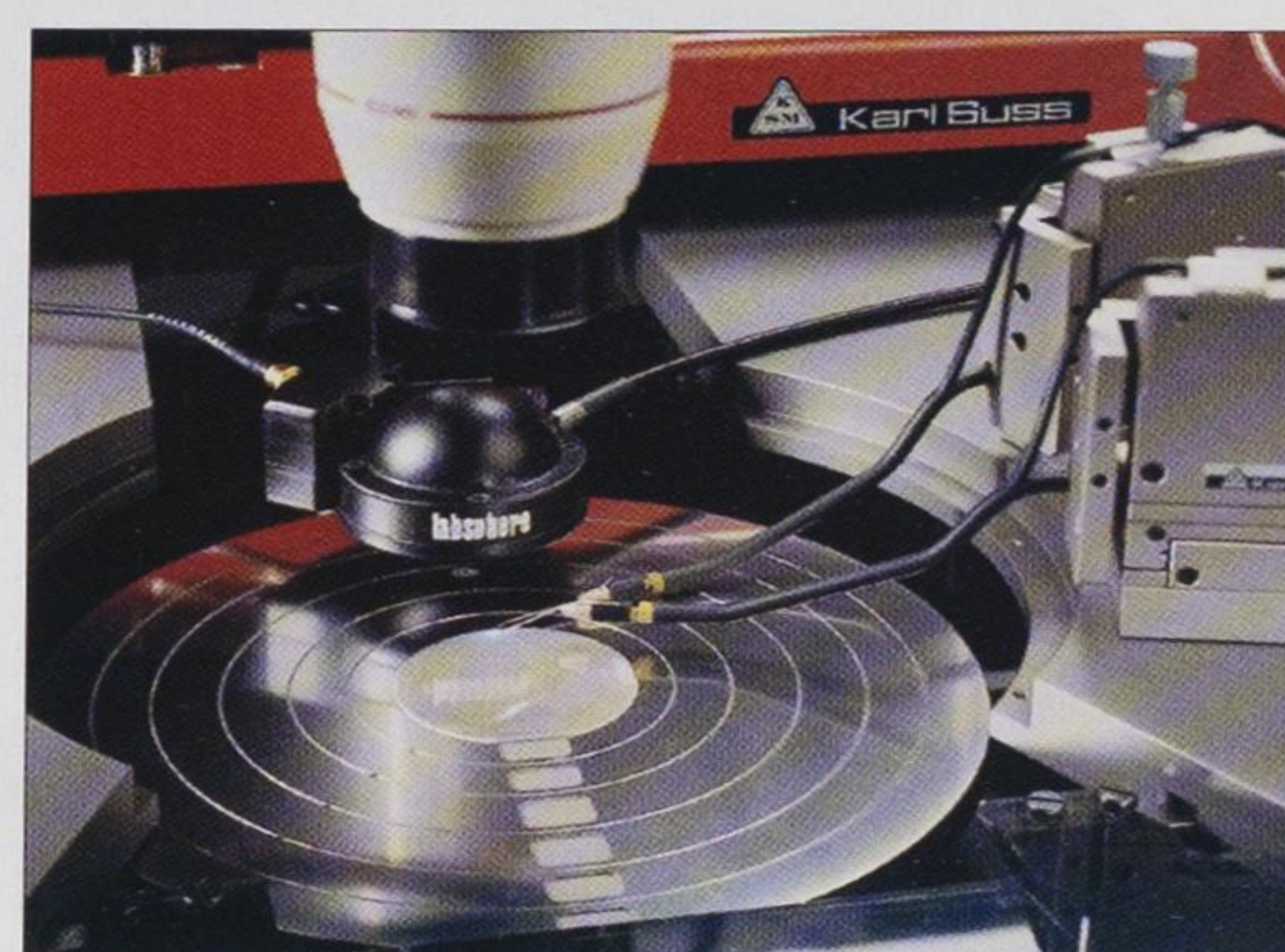
Fig. 1. The wafer probe system from Suss Microtec and Labsphere – shown here testing a blue LED – comprises a Suss Microtec PA200 probe system, along with a Labsphere detector assembly, which includes an integrating sphere detector.
