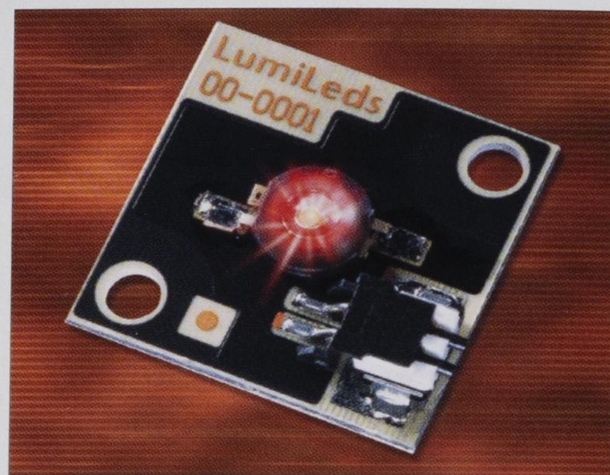
The aluminum heat-sink board is key to the Luxeon LED's high-power operation.
