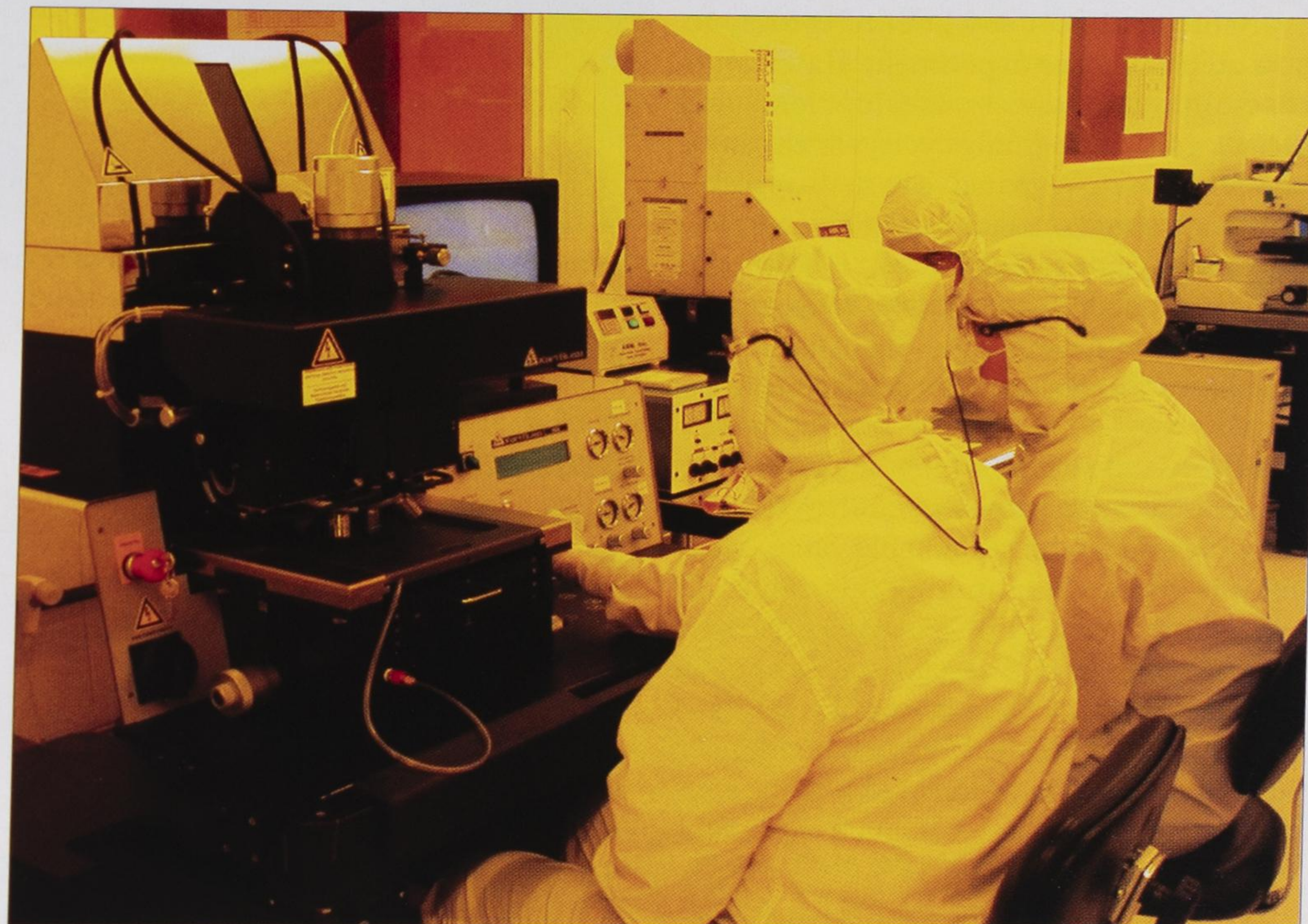
Aligning an InP wafer at VSK Photonics' new fab, which was built in record time.
