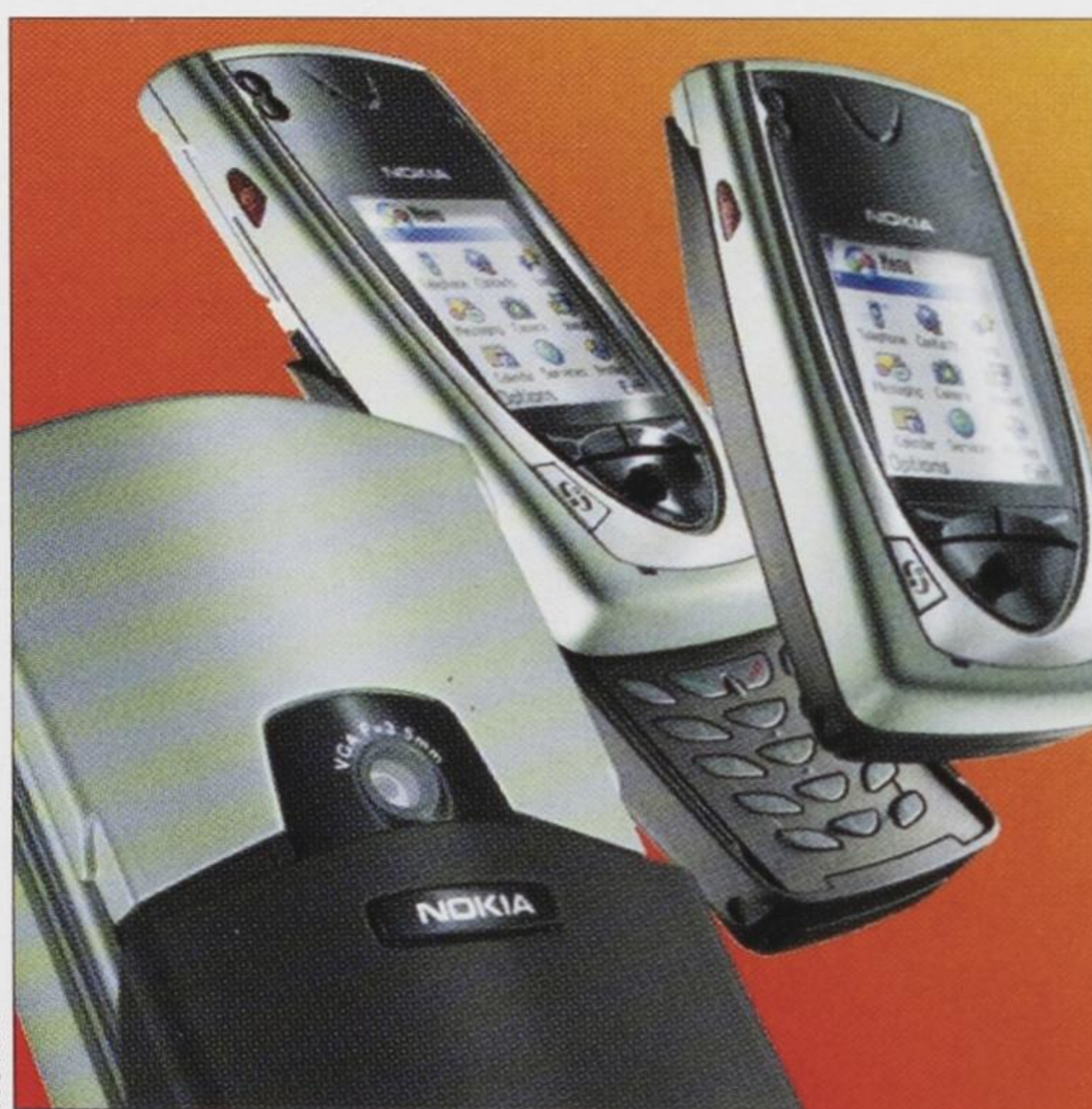
Nokia's new 7650 features a built-in camera with VGA resolution of 640 x 480 pixels, together with a 35 x 41 mm color display.
