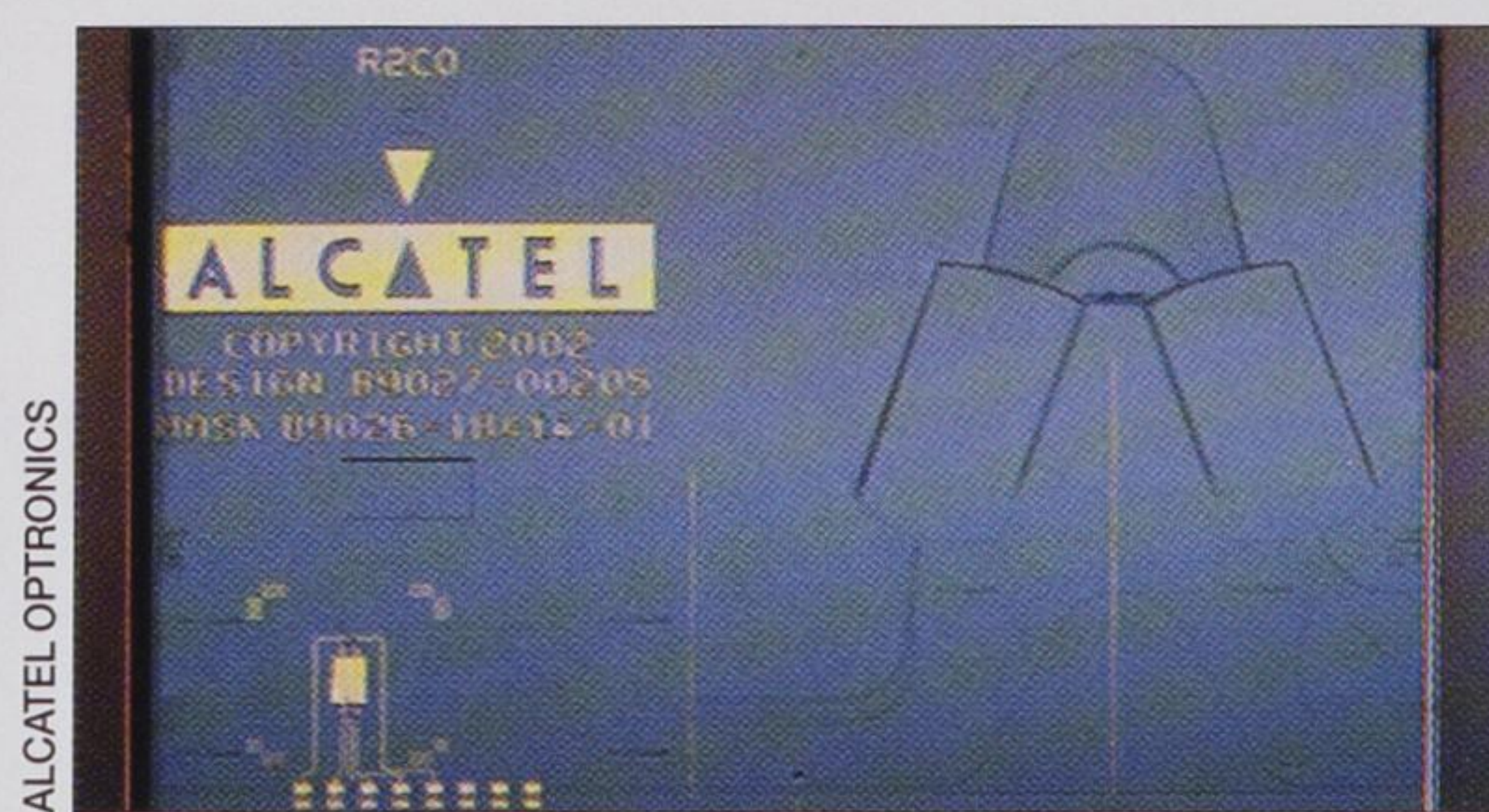
Alcatel Optonics' receiver combines InP-based SOAs (seen at the bottom left of the image) with a silicon-based AWG (seen on the right) on a silica-on-silicon platform.
