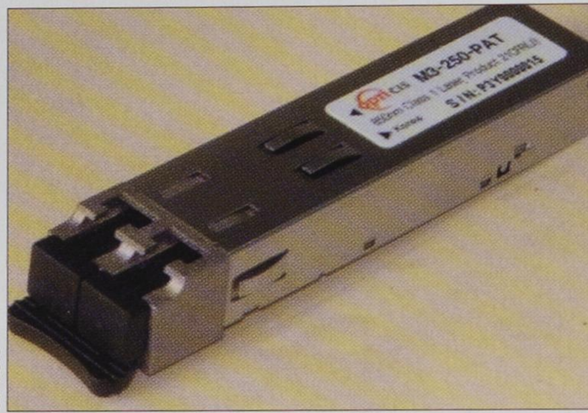
Opticis manufactures transceivers using its own 850 nm VCSELs and pin diodes, so it has tighter control over costs and quality.
