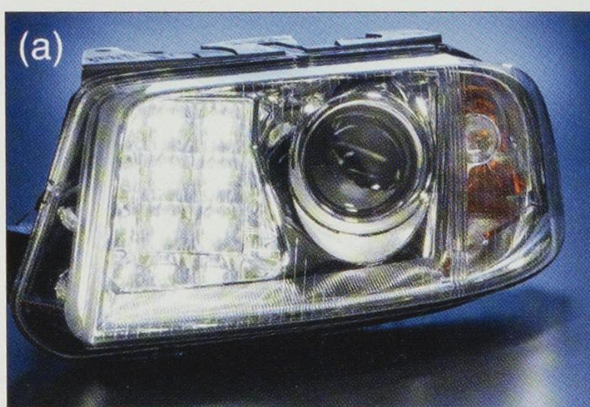
Fig. 4. White LEDs are now being used to provide daytime running lights within headlamps (a), while full headlamp prototypes have also been developed (b).
