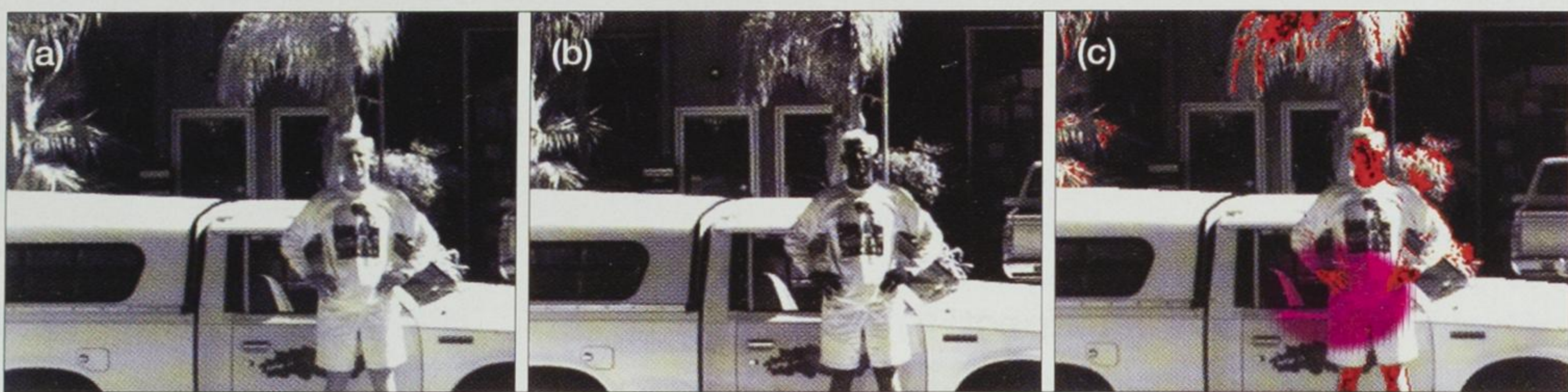
Fig. 4. Image from an InGaAs camera with a 900–1000 nm filter (a) and a 1400–1600 nm filter (b). The third image (c) shows the difference between the other two images, false-colored in red and overlaid onto (a). Exposed skin and vegetation are clearly apparent.
