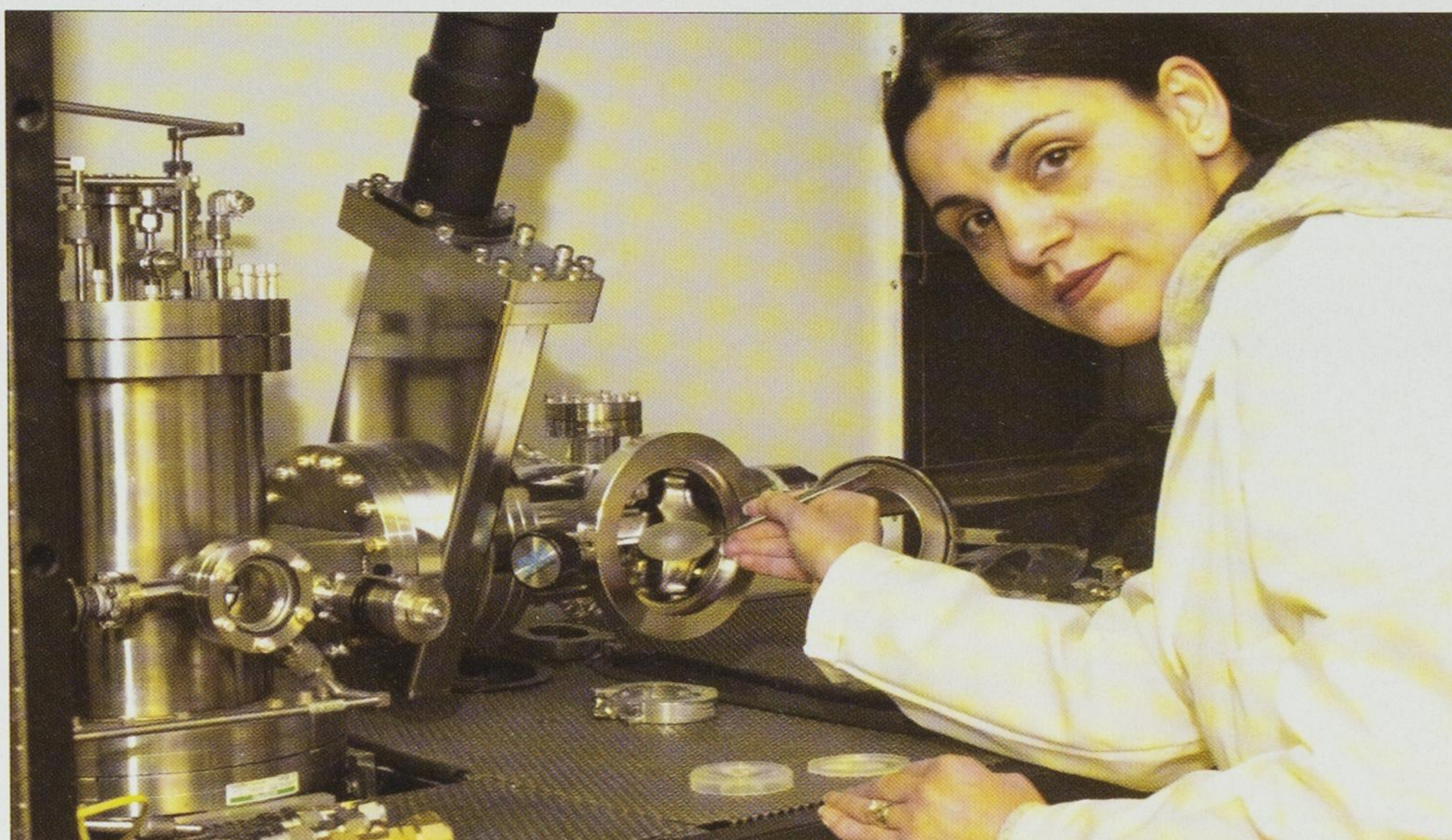
Shadi Shahedipour is leading a team developing GaN-based devices including UV emitters. Growth is done onto sapphire, but the team aims to grow high-quality material on silicon.
