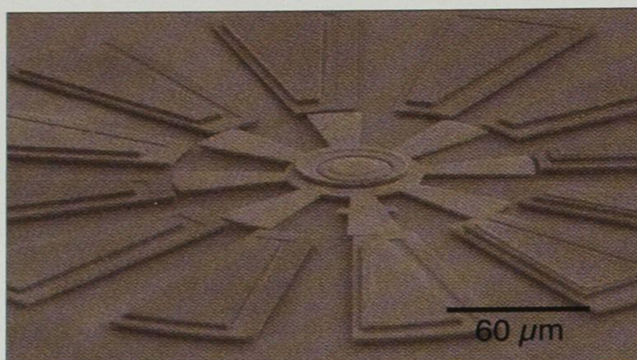
A SiC micromotor produced by FLX Micro during a MUSiC run.
